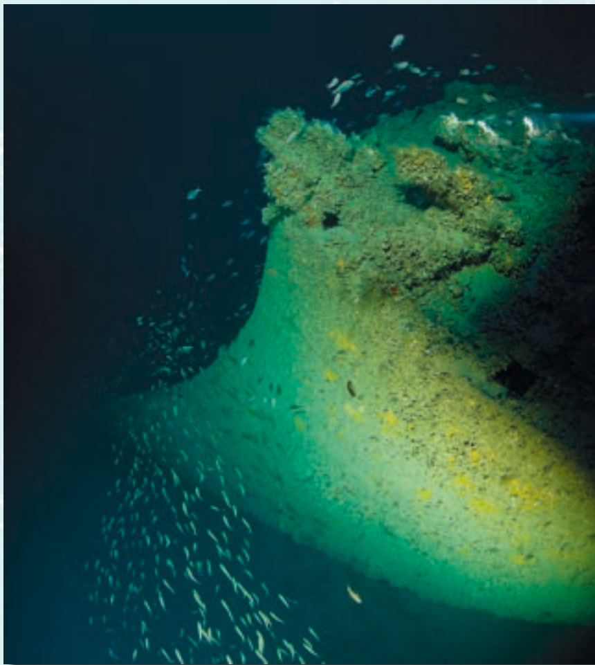
Slika 24, Pramac broda Palestro s kljunom za probijanje Image 24, Prow and battering ram of the Palestro
